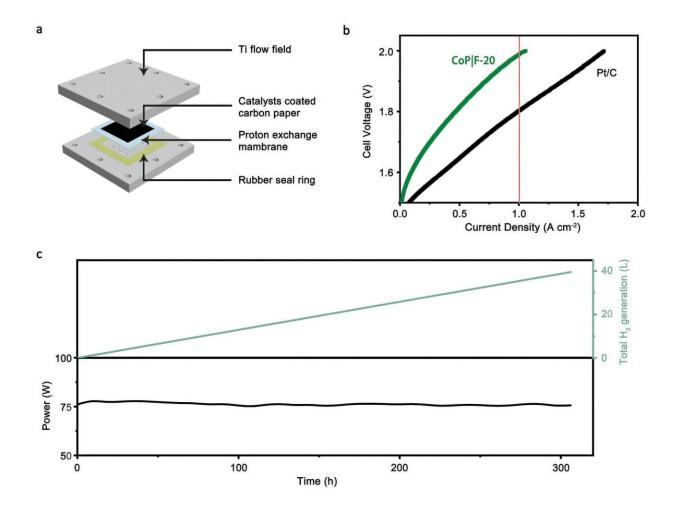
PEM test of CoPlF-20 catalyst. (a) Schematic illustration of a PEM cell. (b) I-V curves of PEM electrolyzers using commercial IrO<sub>2</sub> as an anodic catalyst and CoPlF-20 as a cathodic catalyst. No cell voltages were iR compensated. (c) Time-dependent power and total H<sub>2</sub> generation of PEM electrolyzers using commercial IrO<sub>2</sub> as an anodic catalyst and CoPlF-20 as a cathodic catalyst at 1 A cm<sup>-2</sup>.
