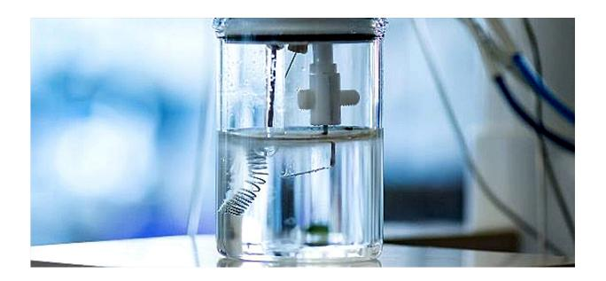
Water electrolysis in action. The double-bent plate at the center served as the electrode material used for electrocatalyst degradation testing in this research. Credit: Ken Sakaushi, National Institute for Materials Science
