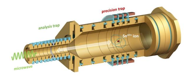
Sketch of the ALPHATRAP Penning ion trap with the precision trap for the measurement of the ion motion frequencies and the analysis trap for spin detection. Credit: MPIK
