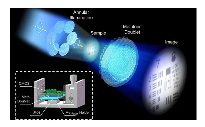
The proposed metalens doublet configuration with annular illumination can overcome off-axis aberrations and achieve unprecedented high-resolution widefield imaging, even in a compact and highly integrated prototype. Credit: Tao Li and Jiacheng Sun (Nanjing University).
