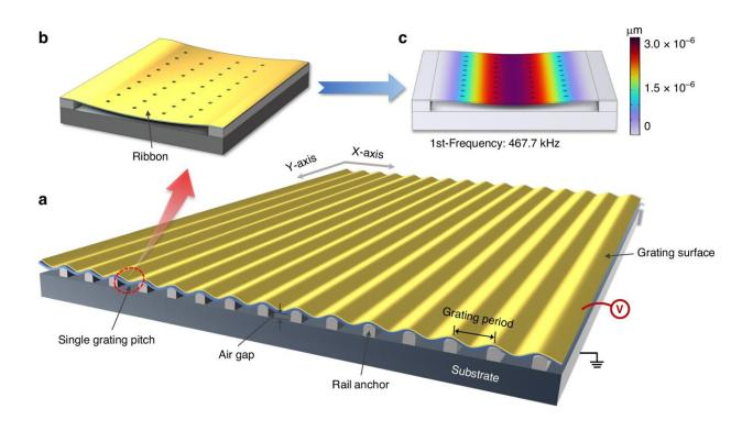
Schematic diagram of the proposed MEMS grating modulator. Credit: *Microsystems & Nanoengineering* (2025). DOI: 10.1038/s41378-025-00894-7
