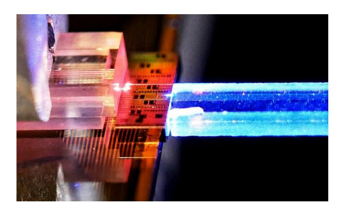
Network IT: A photonic chip coupled to a highly nonlinear crystal and a fiber array unit. The crystal produces entangled visible-telecom photon pairs, which are processed on silicon nitride and silicon photonic integrated circuits enabling a compact and versatile platform to link visibly accessed quantum nodes over existing telecommunications infrastructure. Credit: RIT
