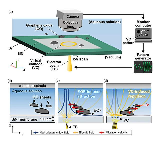
Overview of dynamic graphene oxide sorting: (a) The system uses electron beams on silicon nitride membranes to create electric field patterns that generate
