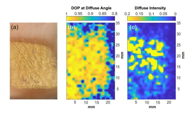
Polarimetric measurements of terahertz scattering can detect subtle changes in tissue architecture that result from disease or damage. For example, terahertz measurements demonstrated signal contrast between burned and healthy skin regions. Credit: *Journal of Biomedical Optics* (2025). DOI: 10.1117/1.JBO.30.6.066001
