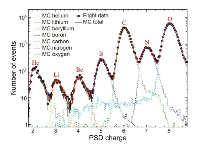
The charge spectrum from DAMPE's PSD for particle identification of cosmic rays. Credit: *Physical Review Letters* (2025). DOI: 10.1103/PhysRevLett.134.191001
