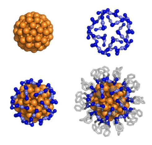
New research shows how gold clusters mimic the key properties of the most accurate systems currently used in quantum applications, showing promise for a tunable, scalable option for quantum devices. The cluster contains a gold core, on top left, as well as ligands, on the bottom right. Credit: Knappenberger Lab / Penn State
