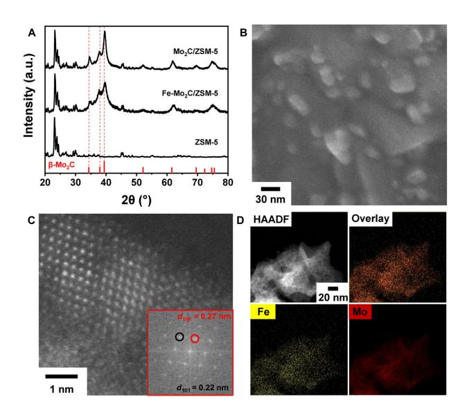
Characterizing the structures of Fe-Mo<sub>2</sub>C/ZSM-5 catalyst.(A) XRD patterns, (B)
