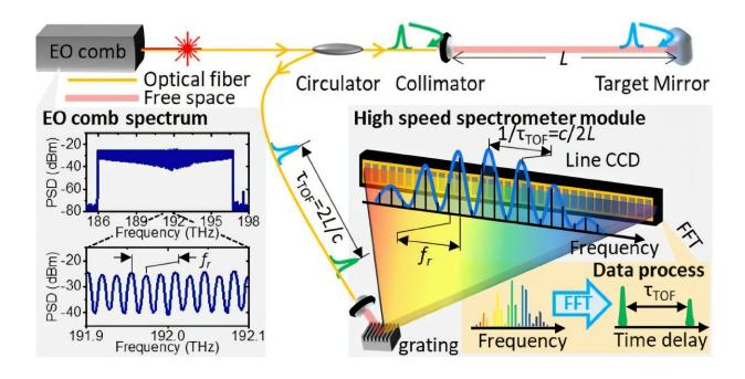
(2-1) Measurement principle of the optical frequency comb-based absolute distance measurement system developed by KRISS. Credit: Korea Research Institute of Standards and Science (KRISS)
