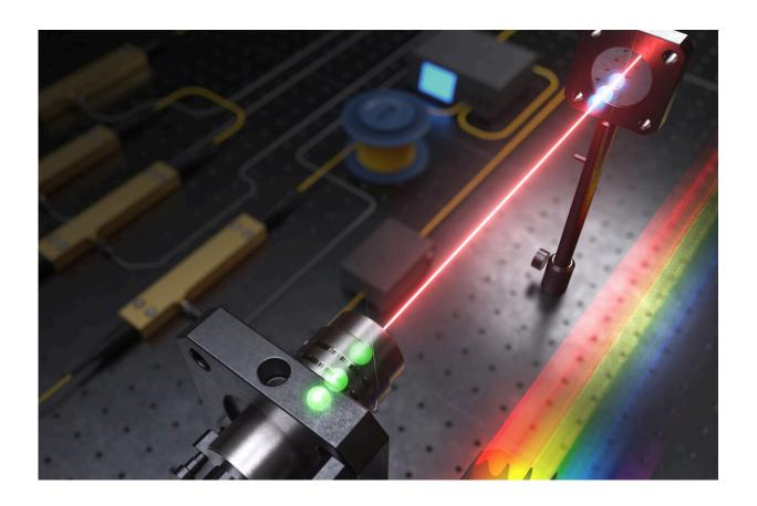
Schematic of the absolute distance measurement system based on the optical frequency comb interferometry developed by KRISS. Credit: Korea Research Institute of Standards and Science (KRISS)
