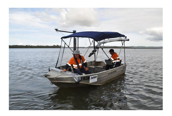
Boats in the Tweed and Richmond rivers with sonar equipment collected accurate information on the cross sections of the river network (river bathymetry) to inform the hydrodynamic model. This also included small remotecontrolled boats for smaller and steeper streams. Credit: CSIRO
