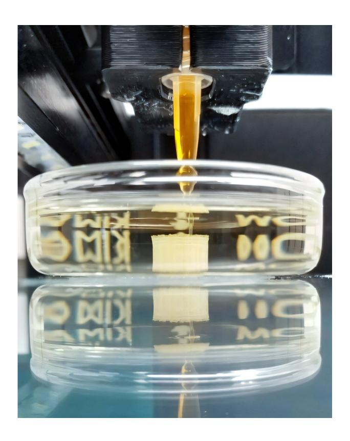
A copolymer-inorganic nanoparticle ink is deposited during the 3D printing process, where it self-assembles before being heat-treated into a crystalline
