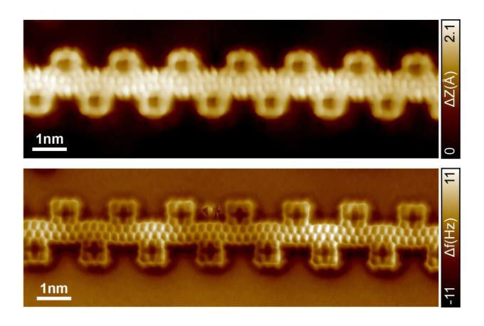
Ultimate precision: With their method, Empa researchers can synthesize the molecular structure with atomic precision, as confirmed by microscopy imaging (top: scanning tunneling microscopy; bottom: non-contact atomic force microscopy). Credit: Swiss Federal Laboratories for Materials Science and Technology
