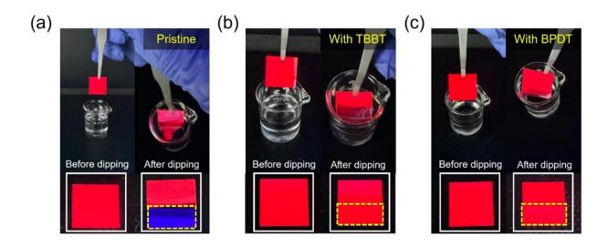
Ligand-crosslinking and solvent immersion test. Photographs of the QD films on silicon substrates for the solvent immersion test: a) Pristine QD film, b) TBBT crosslinked QD film and c) BPDT crosslinked QD film. Credit: *Nano Letters* (2025). DOI: 10.1021/acs.nanolett.5c01926
