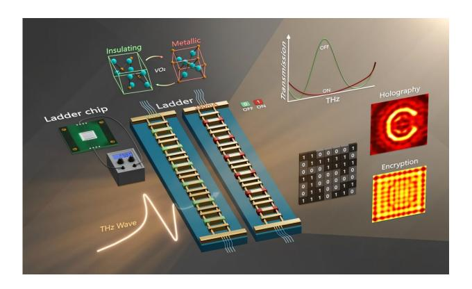
The proposed 'microladder' metasurface has a THz response that can be electrically controlled, making it ideal for holographic imaging and encryption in real time. Credit: Ma, Fan, et al., DOI: 10.1117/1.AP.7.6.066003.
