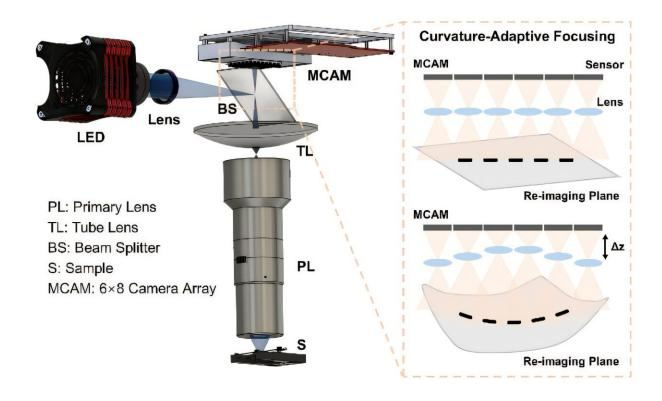
The microscope combines a telecentric lens, a tube lens, and an array of micro cameras, each with its own focus control, making it possible to acquire a seamless, gigapixel image in a single snapshot, flattening out any curvature adaptively. Credit: Haitao Chen, Duke University
