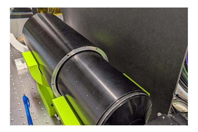
The microscope combines a big telecentric photolithography lens with a large tube lens to create sharp, detailed images of large and curved samples. These lenses project the image onto a flat array of 48 small cameras. Credit: Xi Yang, Duke University
