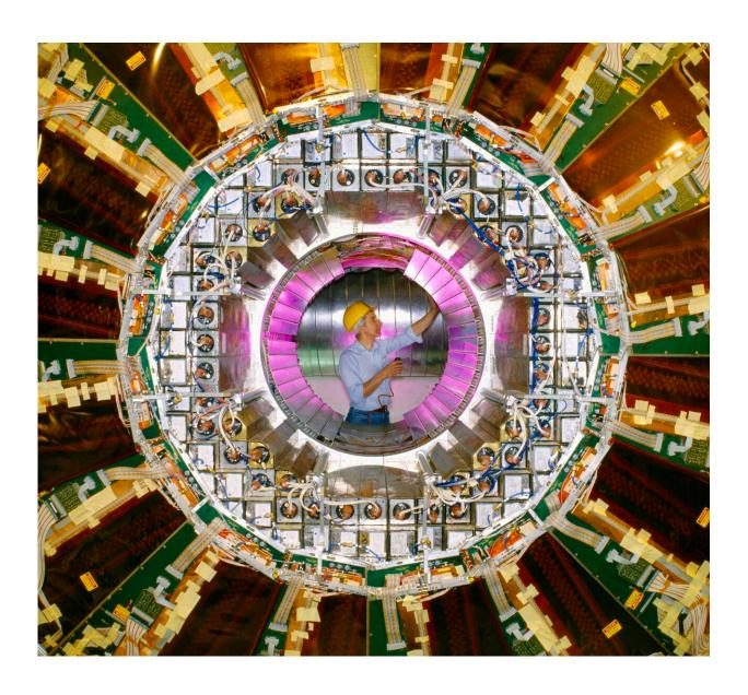
A technician working on the OPAL detector, one of the four particle detectors of the LEP collider. This photo was taken in 1989 and the LEP began running
