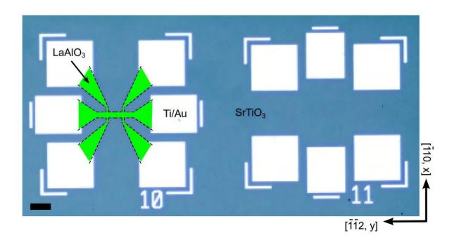
Optical image of two patterned Hall bar devices oriented along orthogonal directions on the  $SrTiO_3$  surface. The green area indicates the position and shape of the devices. Note that the  $LaAlO_3$  layer cannot be distinguished by eye from the substrate. The black scale bar corresponds to 60  $\mu$ m. Credit: *Science* (2025). DOI: 10.1126/science.adq3255
