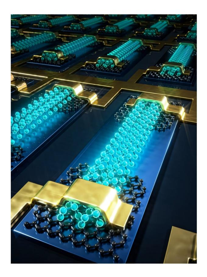
3D scientific illustration of an integrated circuit based on graphene-contacted black phosphorus nanoribbon field-effect transistors. Credit: Changxin Chen Group, School of Integrated Circuits, Shanghai Jiao Tong University.
