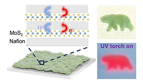
A solid-state PFSA ionomer (Nafion) decouples MoS<sub>2</sub> layers and passivates defects, enabling bright, scalable, stretchable 2D monolayer membranes. Credit: *Journal of the American Chemical Society* (2025). DOI: 10.1021/jacs.5c08388
