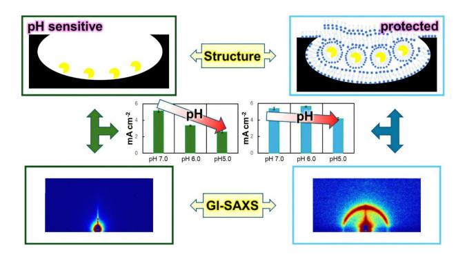
Sucrose monolaurate, when added as a stabilizer to the electrode, formed protective hexagonal and laminar nanostructures around lactate oxidase, shielding it from sweat and maintaining enzyme activity. This, in turn, enabled more accurate lactic acid detection. Credit: Dr. Isao Shitanda from Tokyo University of Science, Japan Image source link: https://pubs.acs.org/doi/10.1021/acs.langmuir.5c02857
