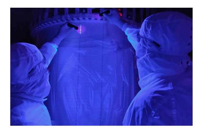
Researchers use UV light to scan for possible dust contamination at the detector's time-projection chamber. Dust can be a source of background noise. Credit: Nicolas Angelides/University of Zurich
