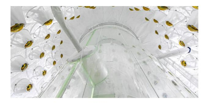
The outer detector of the LZ dark matter experiment. Credit: Matt Kapust/Sanford Underground Research Laboratory
