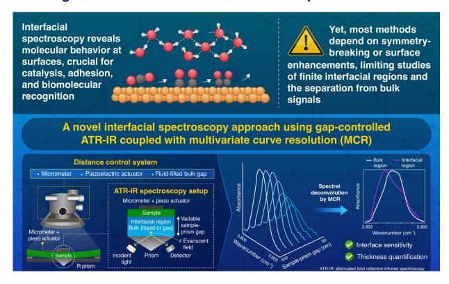
Researchers have developed a low-cost method for the analysis of interfacial molecules by combining ATR-IR with precise gap-control and multi-variate data analysis. Credit: Institute of Science Tokyo
